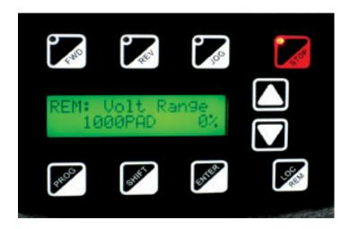
The VFD is capable of handling a wide range of input power. The voltage range for the 230V models is 200-230V +/-10% (180-253V) and for the 460V models is 380-460V +/-10% (342-506V). If input source power is just outside of these ranges, the above screen will be displayed. The VFD is protected from voltage fluctuations within the specified voltage range. Check voltage before plugging in equipment to insure safe operation.
